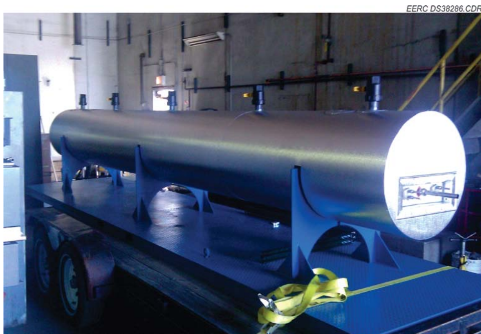
Figure 5. Photograph of pilot-scale anaerobic digester vessel during construction.
